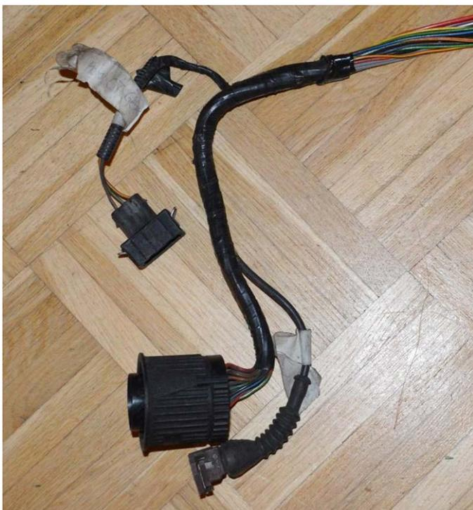
completely stripped loom... some cables must cut off, e.g. some earth or plus cables which are fitted together
